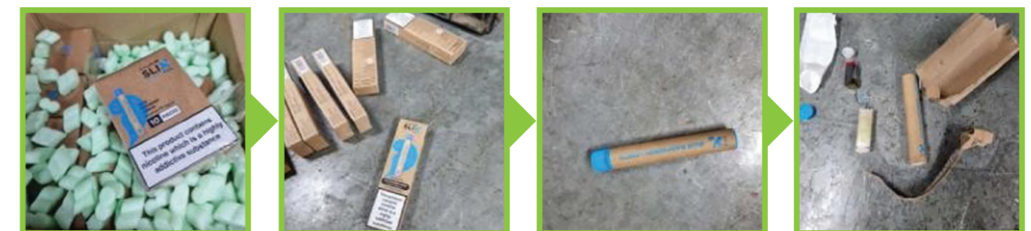
Figure 6. Step by step disassembly of Product B.
