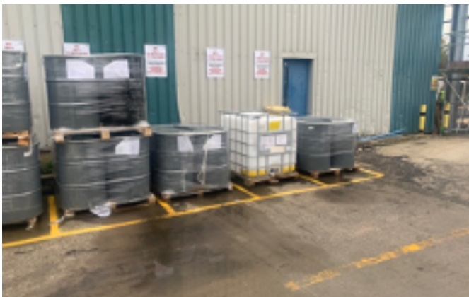
Segregation Area for Hazardous Materials ready for collection
