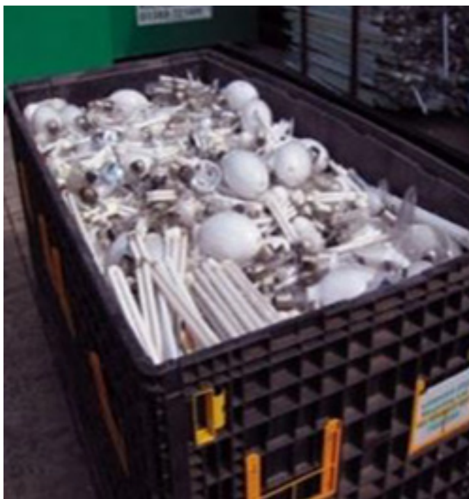
UN approved containers supplied to safely store loose hazardous materials including lamps
